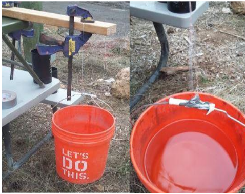
Figure 11: Single Strand Reinforcement Test
