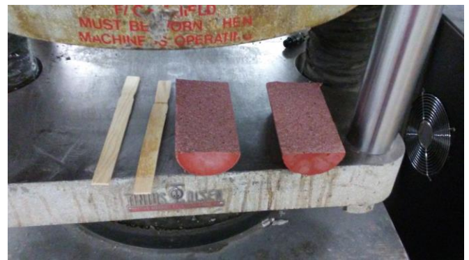
Figure 10: Split Tensile Test
